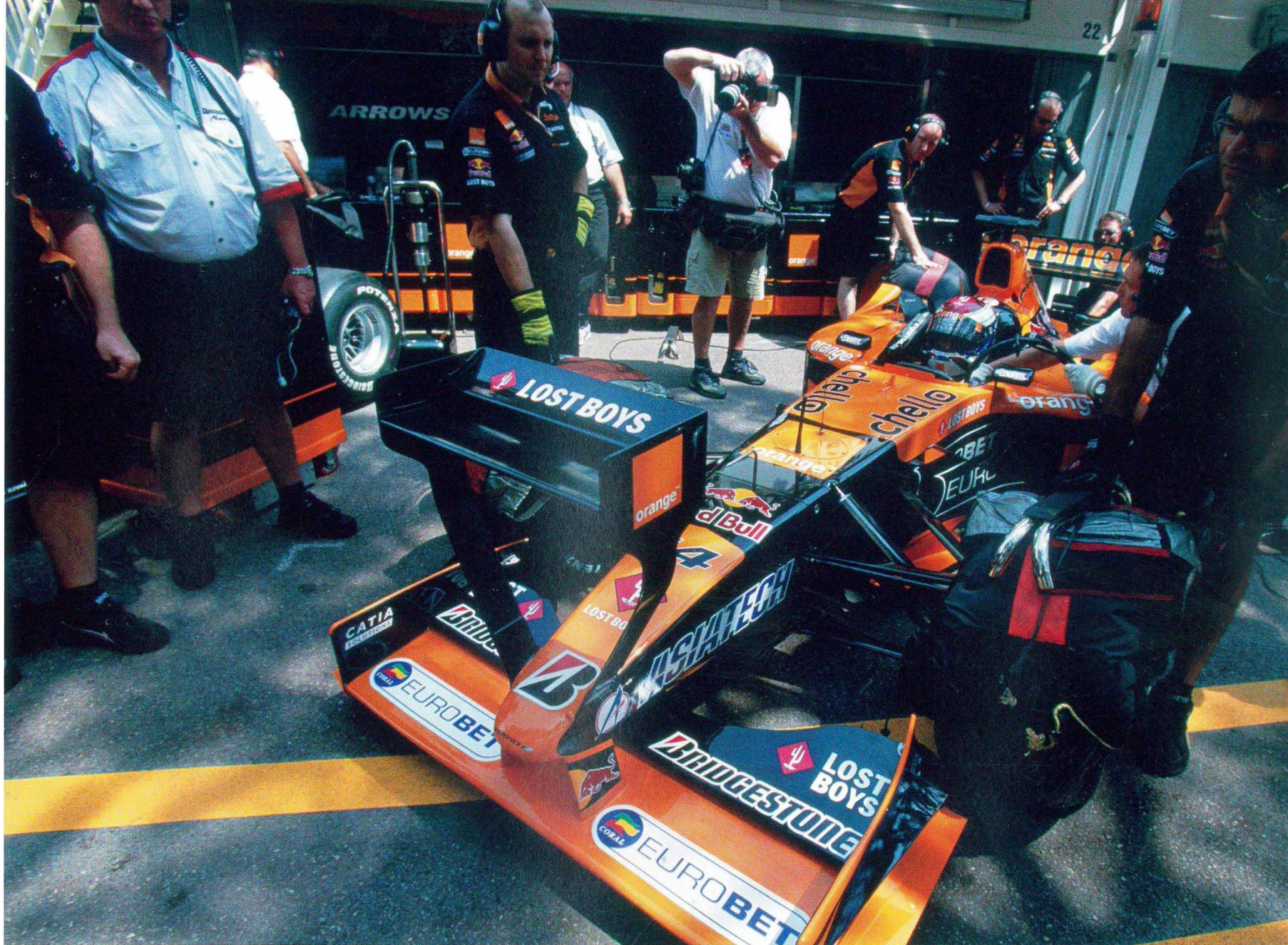
Above: The Arrows A22 of 2001 surprises onlookers at Monaco with this peculiar extra wing mounted above the nose of the car. It was never seen again
